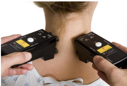
In static sEMG, scanners are held against the body for quick, stethoscope-like measure of muscle tension.
